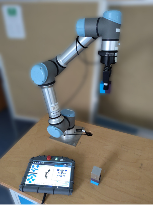
Figure 1. Current setup of the UR5e robot. A 2-finger gripper and a wrist camera are mounted as end effectors. The gripper is holding a block, which should be placed on two other blocks on the table to build a tower. The teaching pendant is placed on the table.
