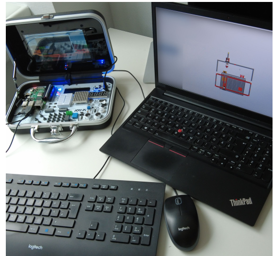
Fig. 1. Experiment setup: On the left side, the Joy-Pi can be seen and on the right side, a virtual three-axis-portal (see [4, Fig. 4]) can be seen.
