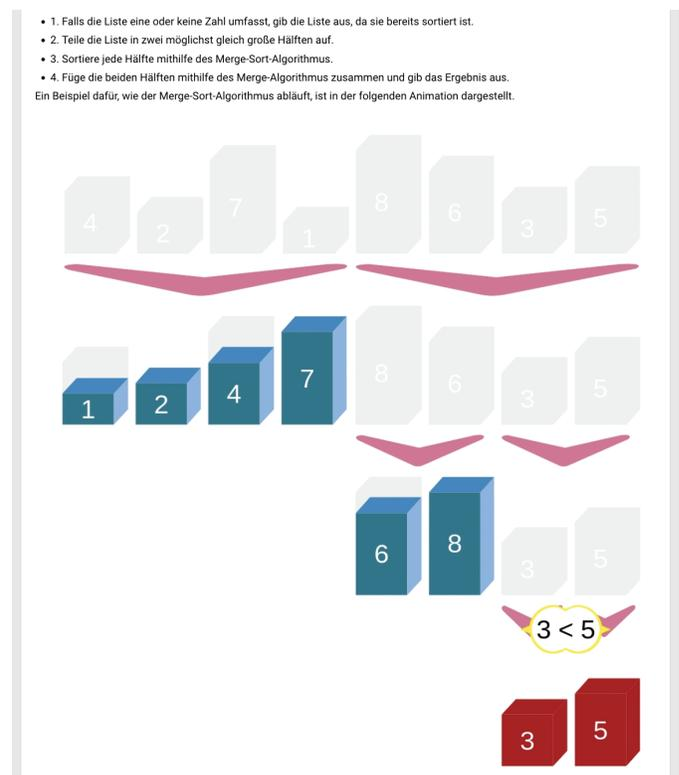
Fig. 1. Example of a GIF in the Algorithm chapter of the MINTFIT computer science course to illustrate the Merge Sort Algorithm.
